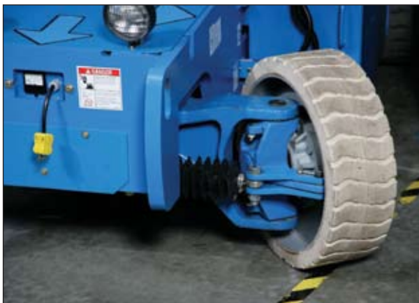
Improved wheel speed control allows for a 57° turning angle.
