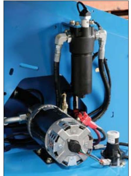
The DC-powered hydraulic system now utilizes a high-pressure filtration system.
