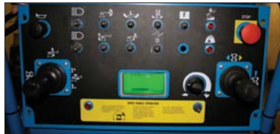
The display screen may be moved inside the upper control box, and a standard Genie battery level indicator may take its place.
